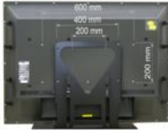
Picture 13 - VESA Standard Mounting Interface
